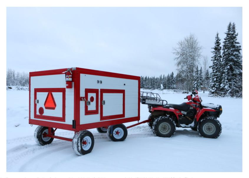
The ThawRig, which is a self contained unit that supports the ThawHead where needed. It houses a generator, electric heater, water pump battery charger, water tank antifreeze storage tank, pressure washer and the ThawHead itself.Photo Courtesy Cameron Gackstetter
